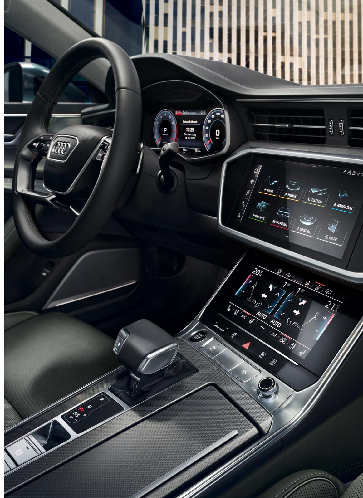
The MMI touch response operating concept offers the benefits of simple, intuitive control in the style of a smartphone and is safe to use even while driving thanks to touch feedback.
